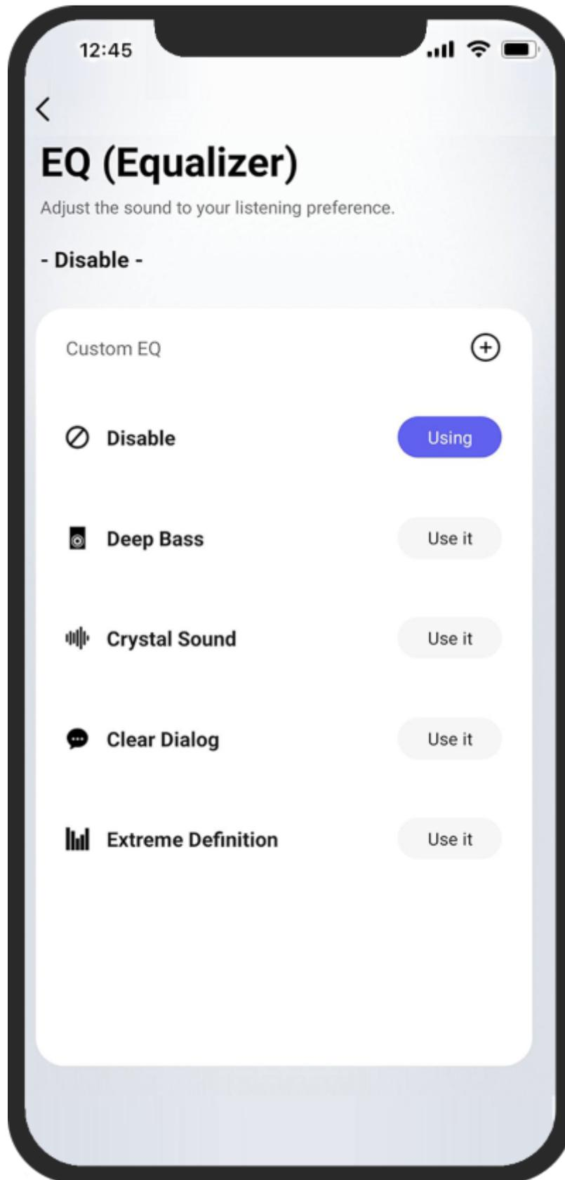
Tapping "+" will take you to a 10-octave band equalizer where you can adjust equalization per band, configuring it to your liking within a range of 24 dB.
